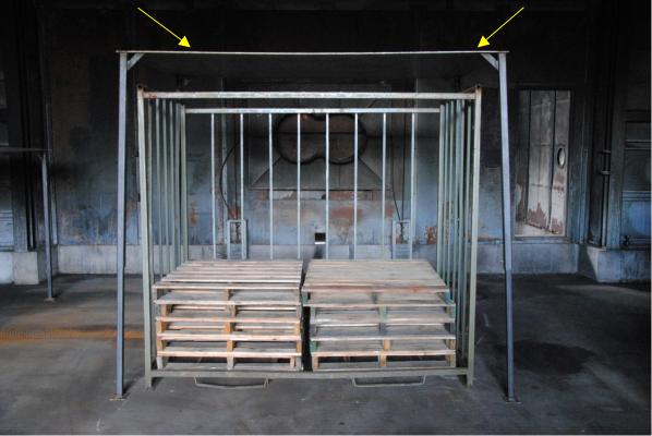
Figure 3: Steel sheeting above the fire load
