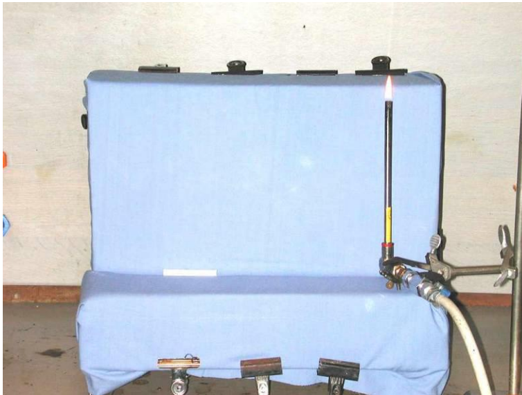
Figure 3 Test setup according to BS5852-1
