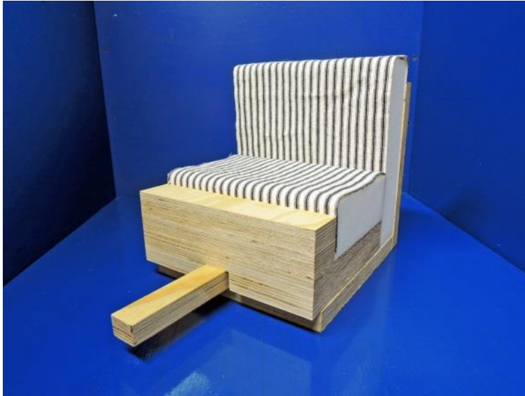
Figure 7 Example of TB117 test set-up
