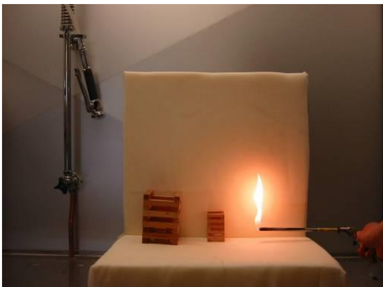
Figure 4 Test set-up for testing according to BS5852-2
