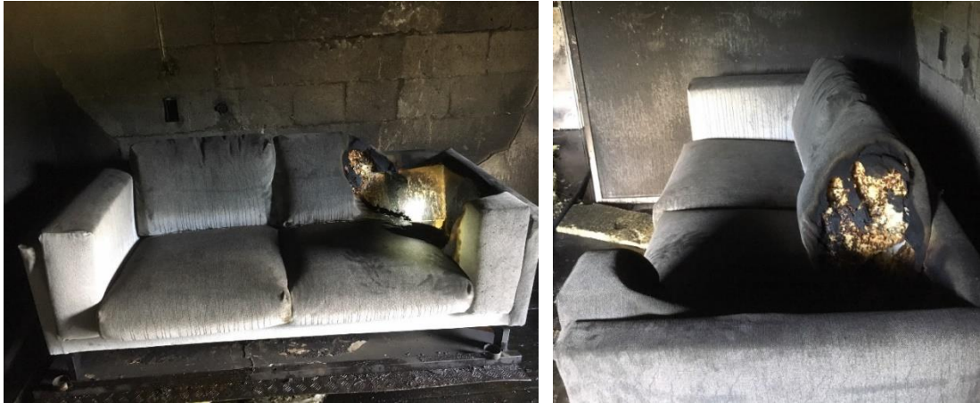
Figure 2.19 Effect smoke-resistant separation and mobile water mist system, offensive interior tactic
