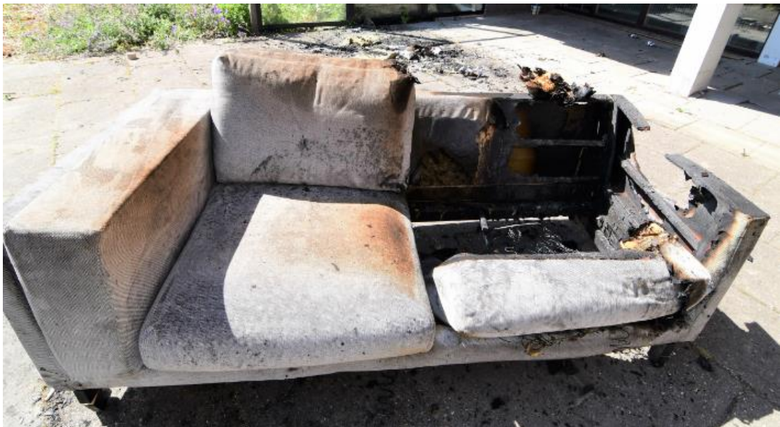
Figure 2.8 Pictures of the sofa after offensive interior attack with door closed
