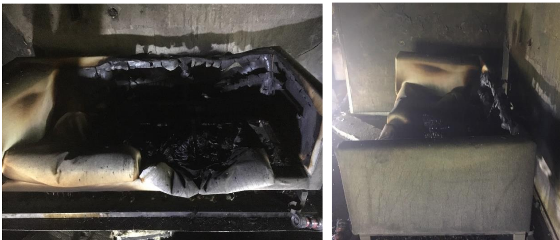
Figure 2.16 Effect mobile water mist system, defensive interior tactic, door open
