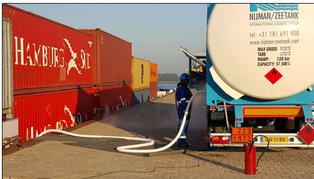
Figuur 2.1 Truck-to-ship bunkering Nijman/Zeetank. (Bron: Nationaal LNG Platform, Marjolein Boer)
