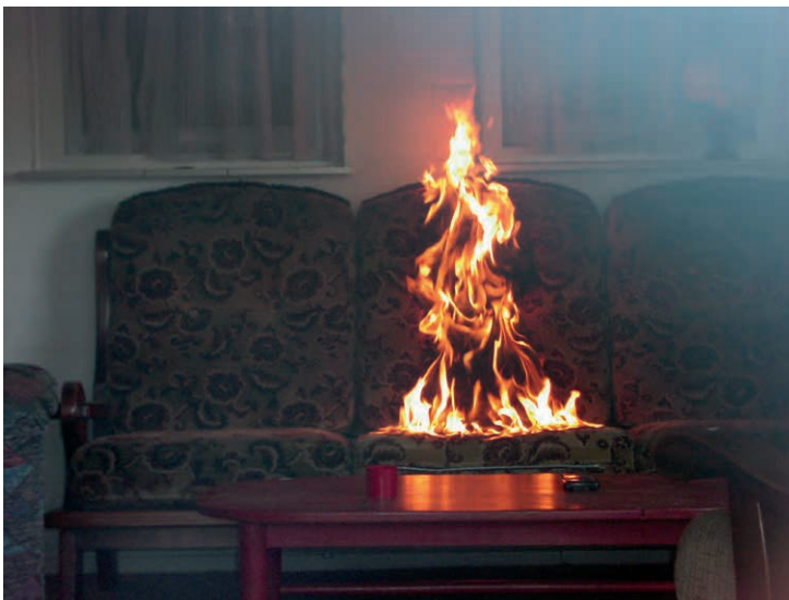
Figure 71 Growth stage of a fire in a room
