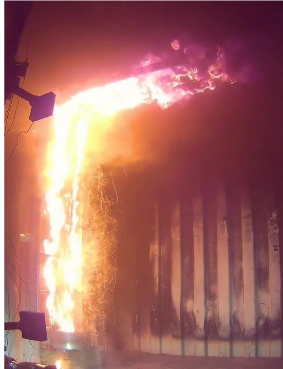
Figure 2.23 Maximum fire size basic performance cables (t = 4:32 min.)
