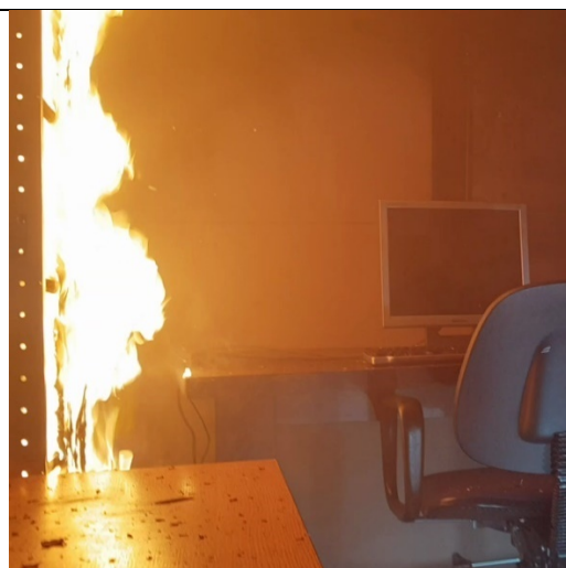
Figure 3.3 After three minutes the desk starts to burn due to heat radiation
