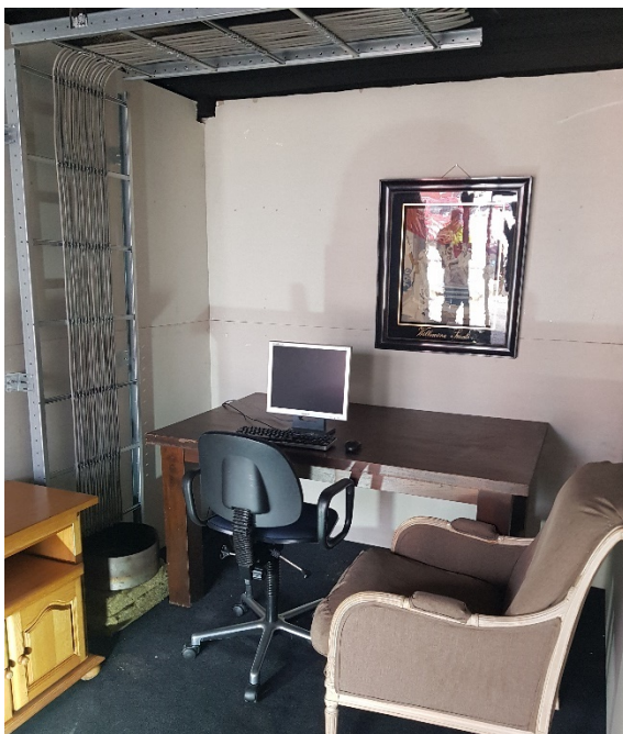
Figure 1.6 Experimental set-up inside the container for the experiment with the basic performance cables in an office environment
