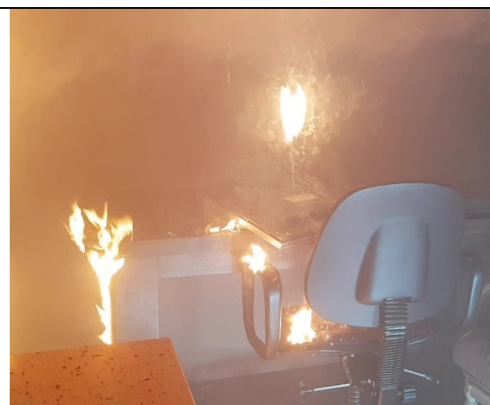
Figure 3.4 After four minutes, burning droplets fall to the floor, desk, monitor and desk chair, allowing the fire to spread
