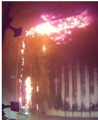
Figure 2.14 4:45 minutes after start test (burning droplets)
