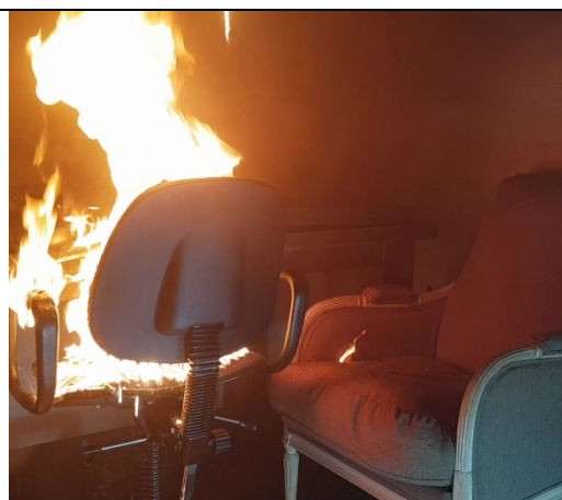
Figure 3.5 After five minutes, more burning droplets fall down causing the armchair to burn
