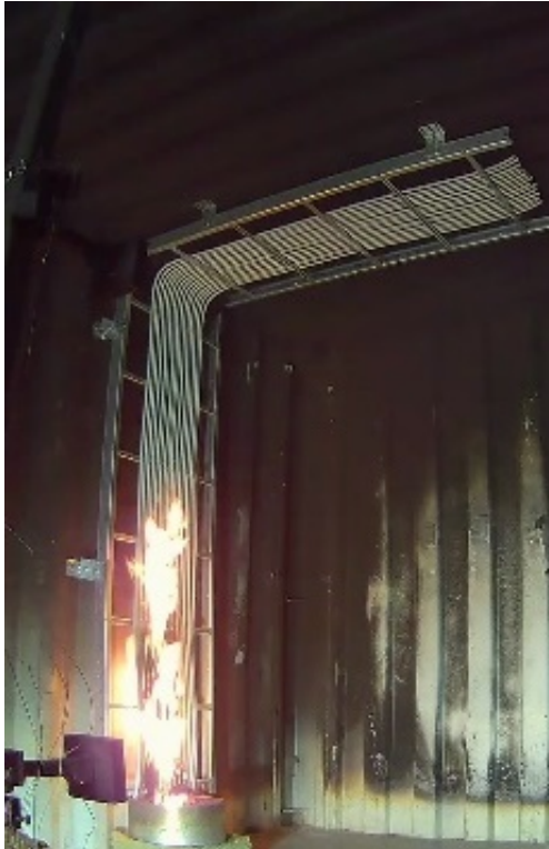
Figure 2.22 Maximum fire size high performance cables (t = 10 min.)
