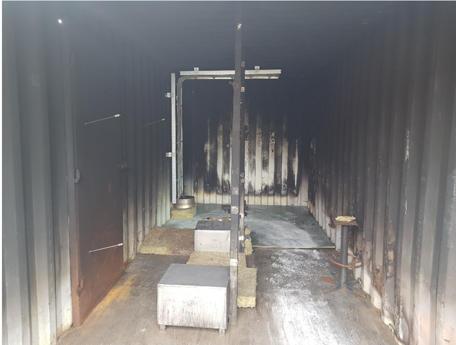
Figure 1.5 Experimental set-up inside the container for the experiments with the high performance and the basic performance cables
