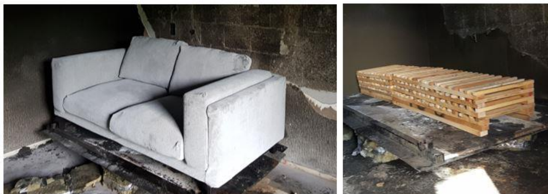
Figure 2.10 Fire objects: sofa (on the left) and organic fire load (on the right)
