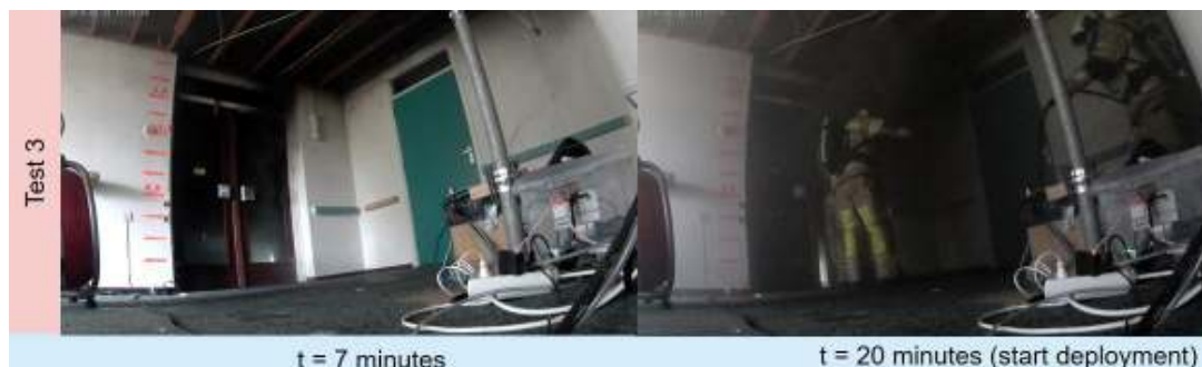
Figure 3.14 Smoke during the escape phase (t = 7 minutes) and the start of the deployment (t = 20 minutes) during test 3 of variant 0
