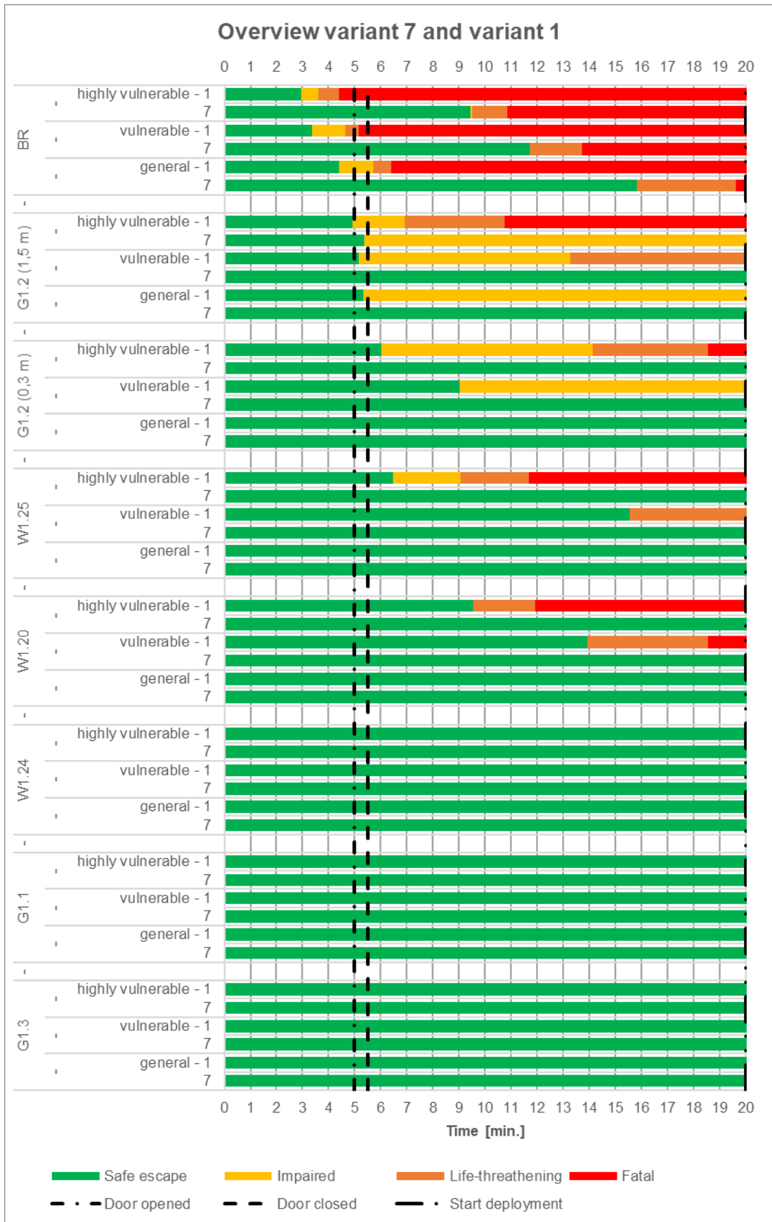
Figure 5.7 Times of the possibility of escape and survivability of variant 7 and variant 1
