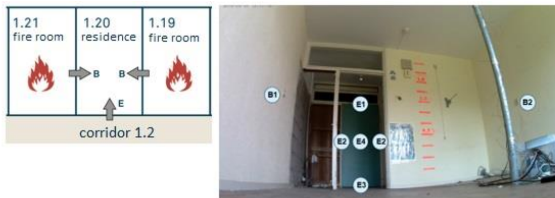
Figure 3.7 Routes B and E, and sub-routes B1, B2, E1, E2, E3 and E4
