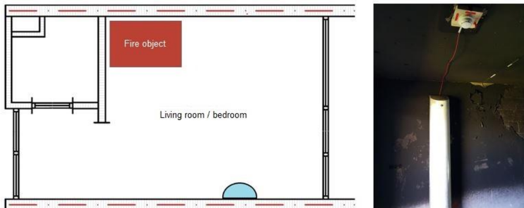
Figure 2.13 Position of the mobile water mist in the fire room and a photo of the mobile water mist
