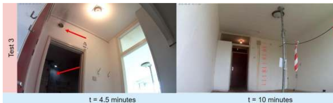
Figure 3.20 Smoke propagation to residence 3.19 via the ventilation ducts during test 3 of variant 0
