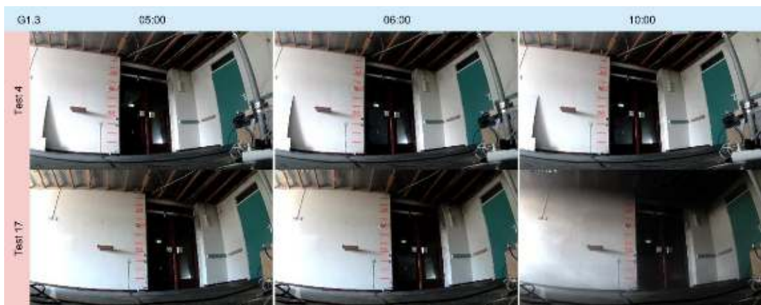
Figure 3.25 Smoke in corridor 1.3 during test 17 of variant 0 and test 4 of variant 1
