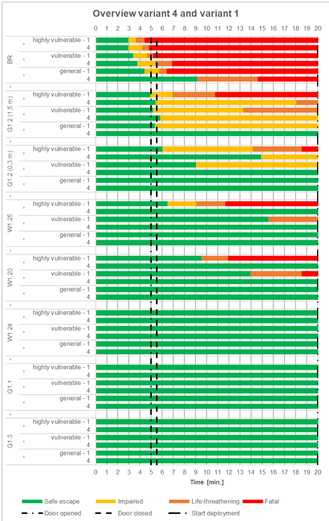
Figure 5.5 Times of the possibility of escape and survivability of variant 4 and variant 1
