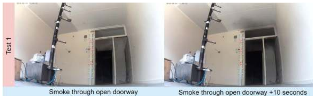
Figure 3.12 Smoke propagation to residence 1.25 after the door to the fire room was opened during test 1 of variant 0
